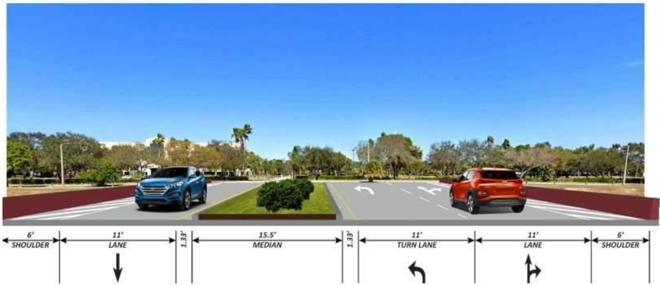
Figure 3-2: Build Alternative 2 Typical Section
